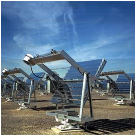
Q-TRAC natural sunlight concentrator testing at Q-Lab Arizona
